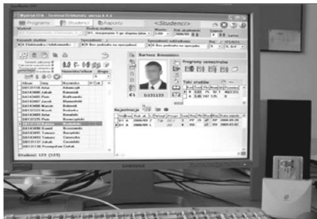
Figure 2: Sample card reader (bottom right) connected to a PC terminal (dean’s office terminal window).
