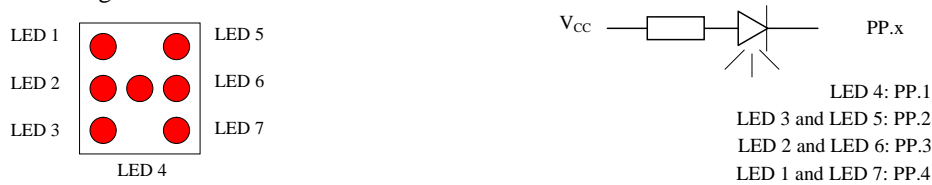
Figure 7: An e-dice comprising seven LEDs driven by four microcontroller parallel port pins.
