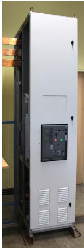
Figure 1: MV switchgear test with switch Entelliguard 2000A (1600A), GE Power Controls.
