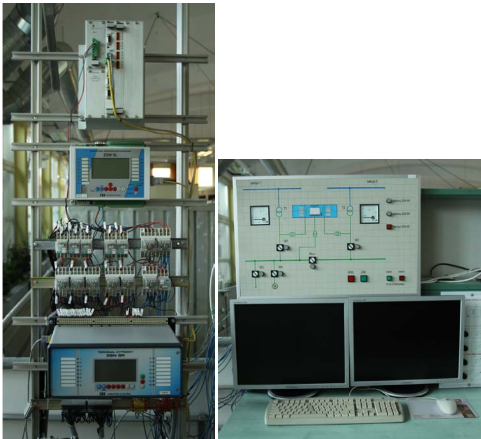
Figure 2: The position measuring system protection type INS 5L.
