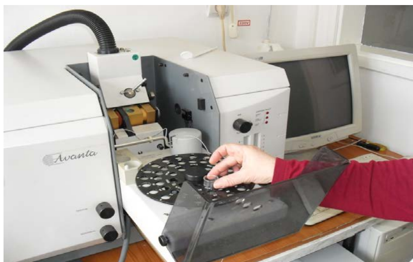
Figure 1: Student loading a sample into the atomic absorption spectrometer.
