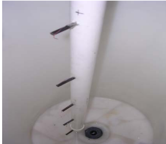
Figure 2: Thermocouples location in the storage tank.
