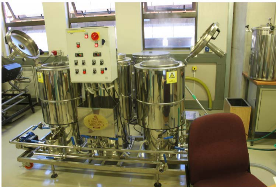
Figure 2: The micro-brewery that needs to be automated.
