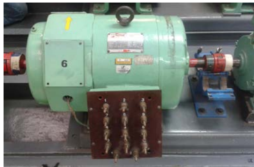
Figure 1: Synchronous machine in the Electrical Machines Laboratory at the National University of Colombia.
