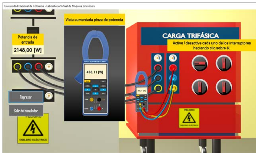
Figure 7: Screen of the efficiency test module against the connected load of the Virtual Laboratory of Synchronous Machines (Source: Authors).
