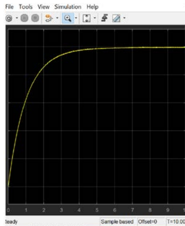
Figure 3: The first order response of the RC circuit.
