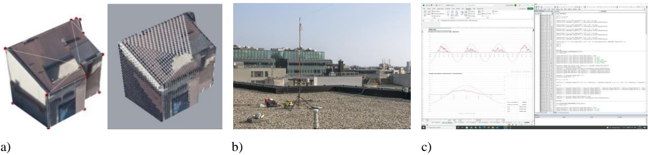
Figure 5: a) automation of the process of determining albedo values of city surfaces through machine learning based on orthophoto maps; b) sensing probe located on the FAD-STU rooftop recording various parameters that influence the formation of urban heat islands, such as the intensity of solar radiation, reflectivity, rate of evaporation, etc; and c) example of recorded measurement dataset (Figures: the authors).
