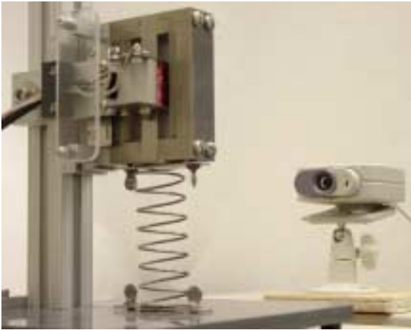
Figure 6: Remotely accessible mechanical vibration set-up with video monitoring.
