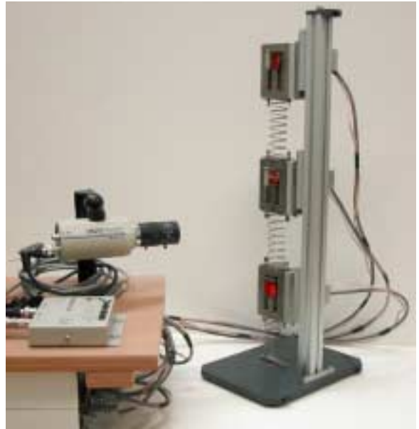
Figure 7: Modular mechanical vibration set-up with multiple degrees of freedom.
